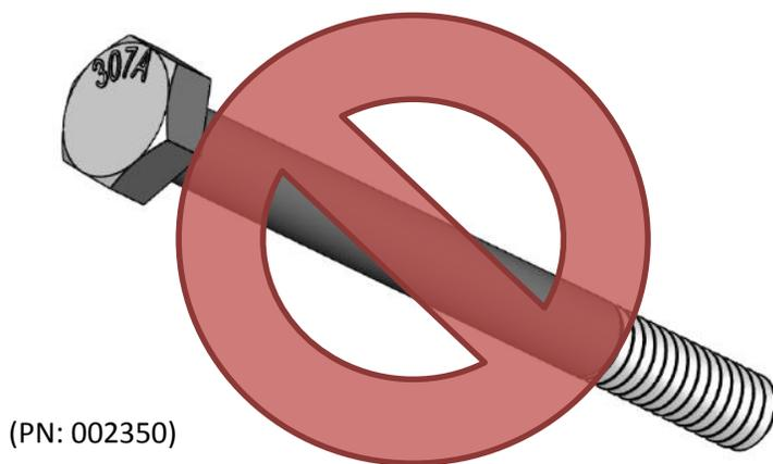
*Figure 1: Diagram illustrating the head markings of a Grade 2 bolt. This shear bolt has been replaced.*
