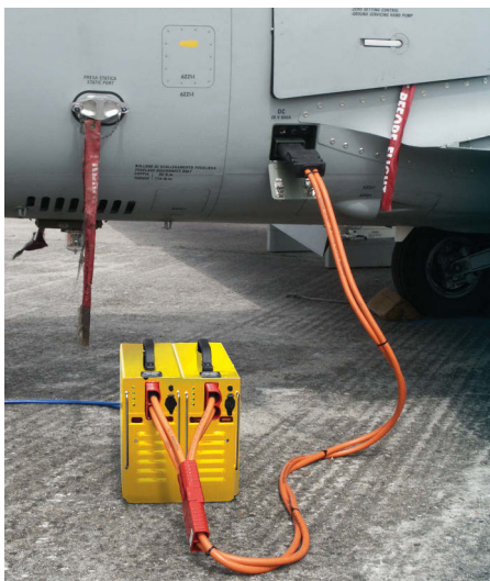
2 x PS100 in parallel: delivering up to 200 amps
