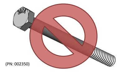
Figure 1: Diagram illustrating the head markings of a Grade 2 bolt. This shear bolt has been replaced.
