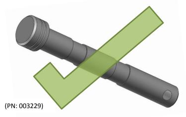
*Figure 2: Diagram illustrating the head markings of a SP2 shear pin. This shear pin takes priority over the Grade 2 bolt.*
